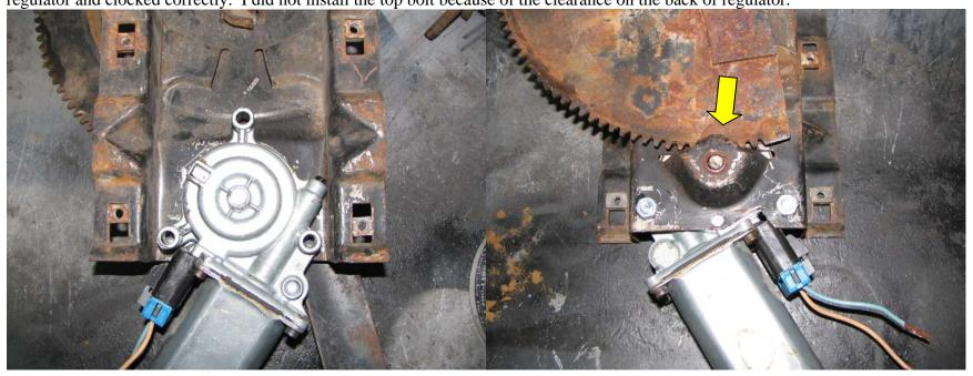
Notice the Yellow arrow? When motor is fully installed you will need the motor teeth matched up to regulator teeth.
